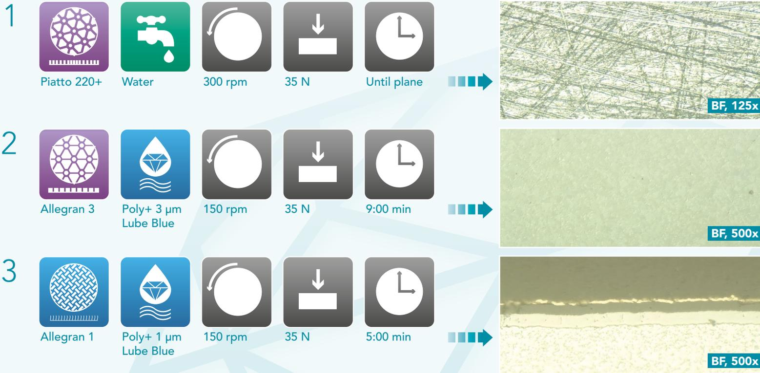
Times are stated for a 300 mm preparation system and Forces for an individual 40 mm dia. sample.
